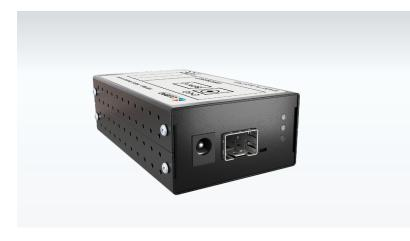
Cubro Media Converter provides seamless integration of copper and fibre, and different fibre types in Enterprise LAN networks. It supports a wide variety of protocols, data rates and media types to create a more reliable and cost-effective network. SFP - SFP Media converter combines data rate and provides independent connectivity with support for SFP and SFP+ transceivers.
